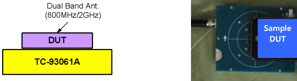
<Figure 4. Place a DUT on the Antenna Coupler- Reactive Field >
